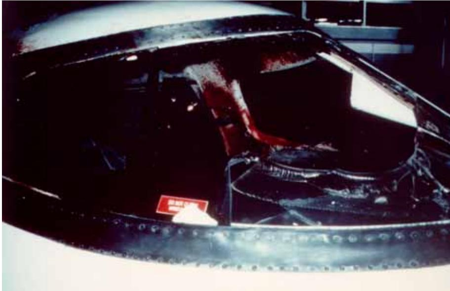
While climbing through 4,000 ft in a left turn, a **Loon** (*Gavia immer*, 3.7 kg) penetrated the right windshield killing the co-pilot and seriously injuring the pilot. Windshield debris damaged engine 2 which had to be shut down. Loss of hydraulics resulted in the flaps and brakes being inoperative. Wind-blast caused communication difficulties. The injured pilot demonstrated a high standard of airmanship in successfully returning to Lunken Airport.
