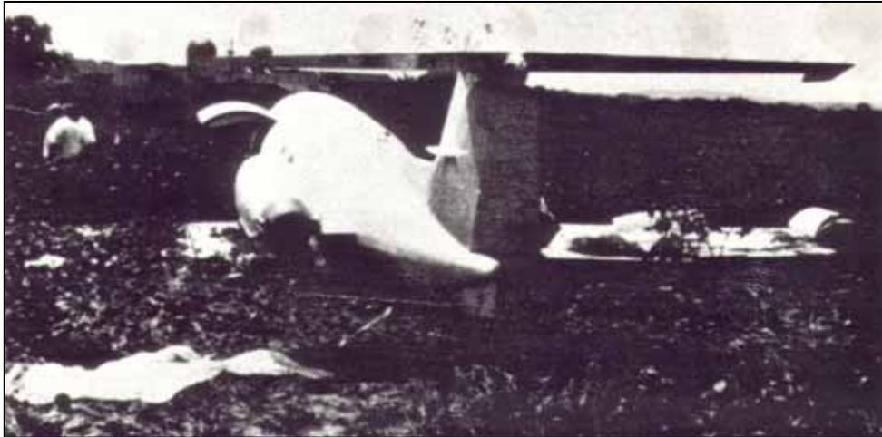
At 500 ft after take-off, the aircraft passed through a flock of 200 **Starlings**, (*Sturnus vulgaris*, 80 gm). Both engines failed and the aircraft force landed, struck a tree between industrial buildings and bounced across a road into a field. There was no fire. The pilot reported it was only 10 seconds from the bird encounter to ground impact.
