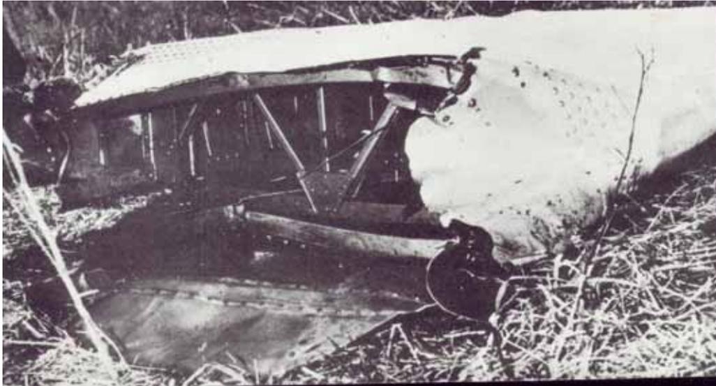
While the United Airlines flight was in the cruise at 6,000 ft en-route from New York, Newark to Washington at night, the aircraft struck **Whistling swans** (*Cygnus columbianus*, 6 kg). Two were struck, one holed the leading edge of the tailplane and exited from the rear surface damaging the elevator, weakening the structure causing the tailplane to detach and the aircraft to crash. As a result of this accident aircraft tail areas are now required to withstand impact with a 3.7 kg bird.
