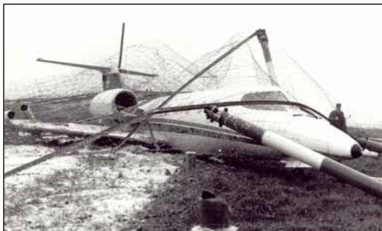
As the aircraft was taking off on a wet runway, a flock of **Black-headed gulls**, (*Larus ridibundus* 275 gm) was encountered when the speed was above V1. Take-off was abandoned and the aircraft over-ran the runway by 56 metres into the ILS installation, which
