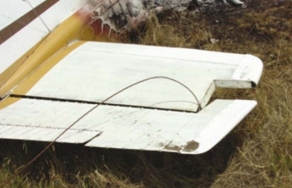
Section of the struck powerline caught in the horizontal stabiliser
