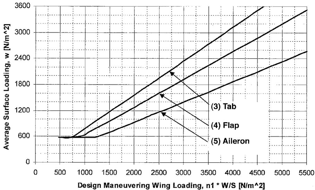
FIG. X1.5 Average Limit Control Surface Loading
