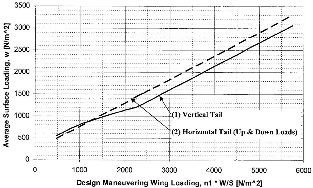
FIG. X1.4 Average Limit Control Surface Loading
