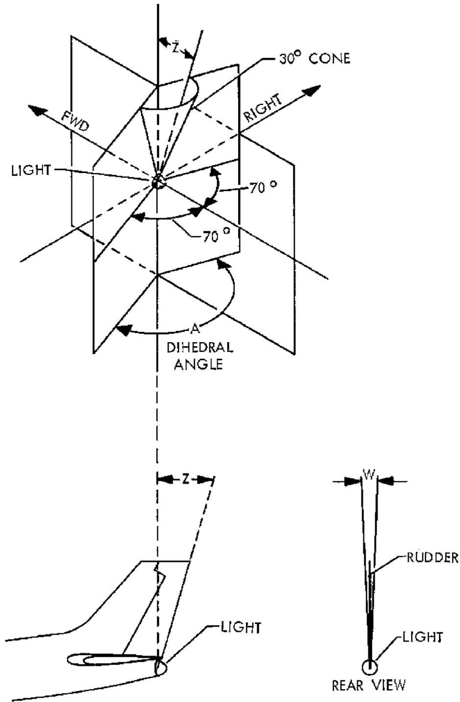
NOTE 1—On the side view drawing, draw a line through the light center perpendicular to the aircraft longitudinal axis. Draw a second line upward through the light center to the most aft point on the vertical stabilizer. The angle  $Z$  between the two lines is limited by the airworthiness rules to  $30^\circ$ . Fig. A2.1 shows an example of angle  $Z$ .
