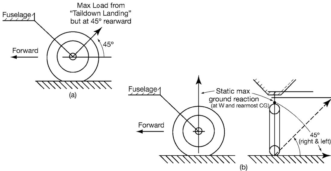
FIG. 5 Supplementary Conditions for Tail Wheel
