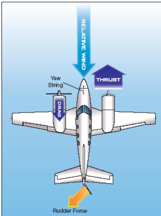
Figure 5: OEI with a Windmilling Propeller Asymmetric Drag
