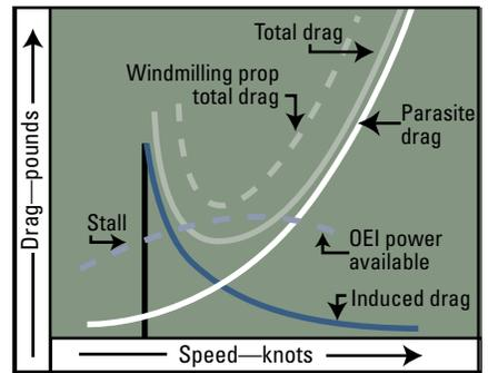
Figure 6: OEI with a windmilling propeller drag and power effects
