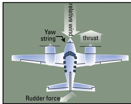
Figure 5: OEI with a windmilling propeller asymmetric drag
