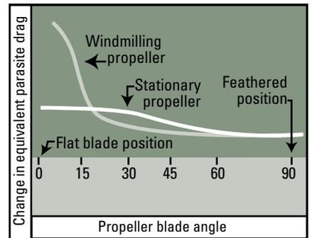
Figure 3: Windmilling propeller parasitic drag
