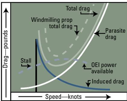
Figure 4: Windmilling propeller total drag
