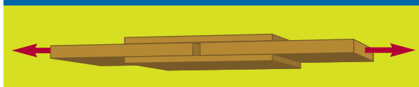
Above: Old fashioned furniture joints are unsatisfactory; aircraft require properly designed joints which put the glue in shear.
